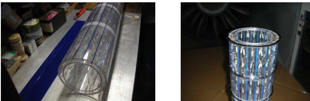
Figure 5 a) b): Model of Solar Updraft Tower: application of surface roughness and stiffening rings.
