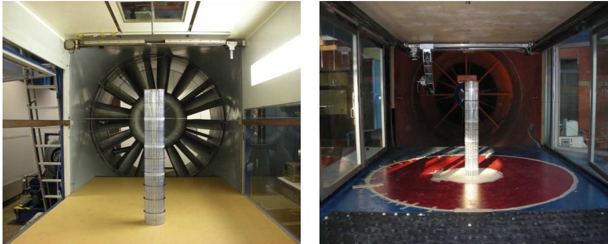
Figure 4: Wind tunnel tests on Solar Updraft Tower. a) WiSt boundary layer wind tunnel, Ruhr-University Bochum, Germany; b) Criaciv boundary layer wind tunnel, Florence, Italy
