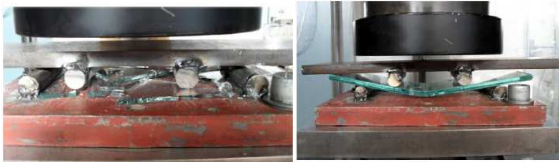
Fig. 7 Bending tests: a) monolithic glass specimen; b) laminated glass specimen (Campione et al. [4]).
