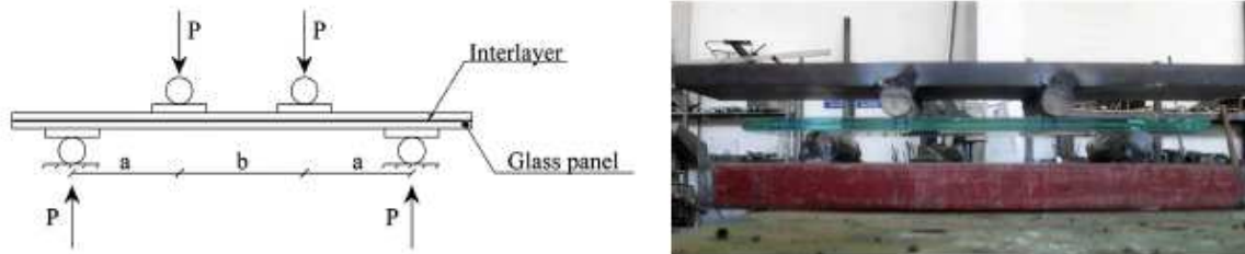
Fig. 5 - loading scheme for flexural tests (Campione et al. [3]).
