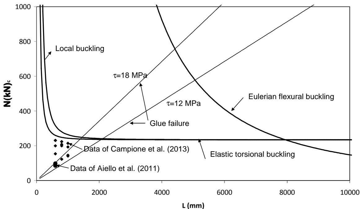
Fig. 2 – Variation of critical flexural load with length variation for T cross-section.
