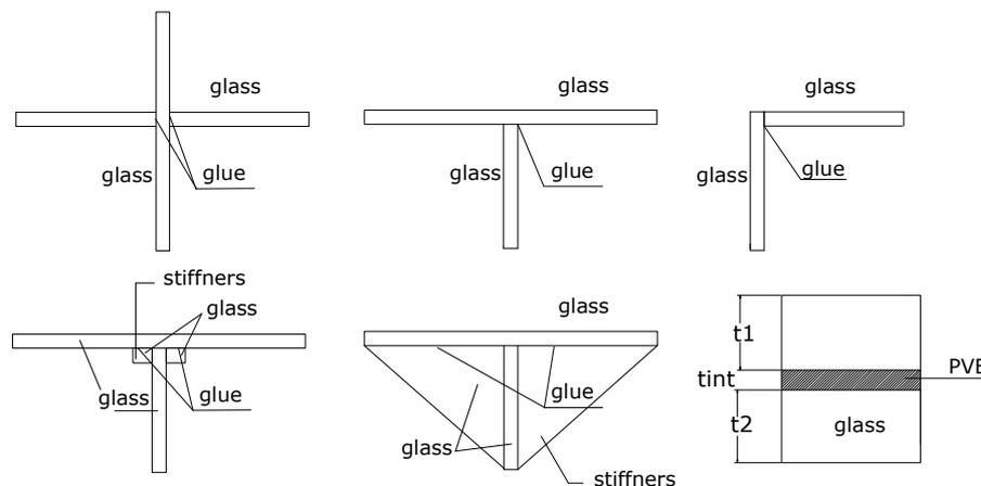
Fig. 1 – Multilayered glass panel and glued connection in different cross-sections.
