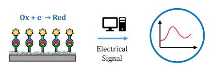
The electroactive tag, for example an enzyme, catalyse a redox reaction generating a detectable electrical signal that can be linked to analyte concentration through a calibration curve.
