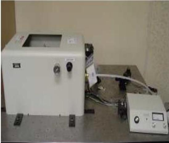
Prism coupling system made by Metricon able to measure thin films refractive index (accuracy  $\pm 2 \times 10^{-4}$ ) and thickness (derived using the Wentzel-Kramers-Brillouin approximation).
