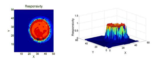
Photoresponse scan of an experimental dye sensitized solar cell via LBIC measurements
