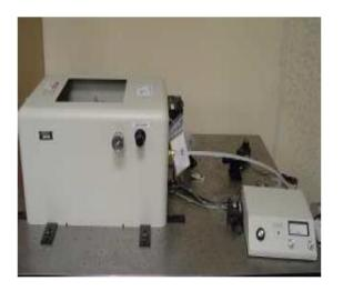
Prism coupling system made by Metricon able to measure thin films refractive index (accuracy  $\pm 2x10^{-4}$ ) and thickness (derived using the Wentzel-Kramers-Brillouin approximation).
