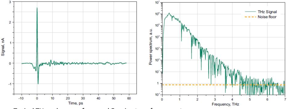
Typical THz pulse waveform and Fourier-transform spectrum
