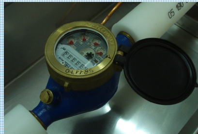
Class C; Q_3 = 2.5 \text{ m}^3/\text{h} ; DN 20 mm
