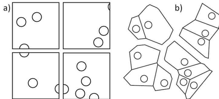
Figure 2: a) Square partitioning at partition scale,  $\delta=5$  b) Similarly sized grouping of cells using Voronoi tessellation partitioning,  $\delta=5$ .
