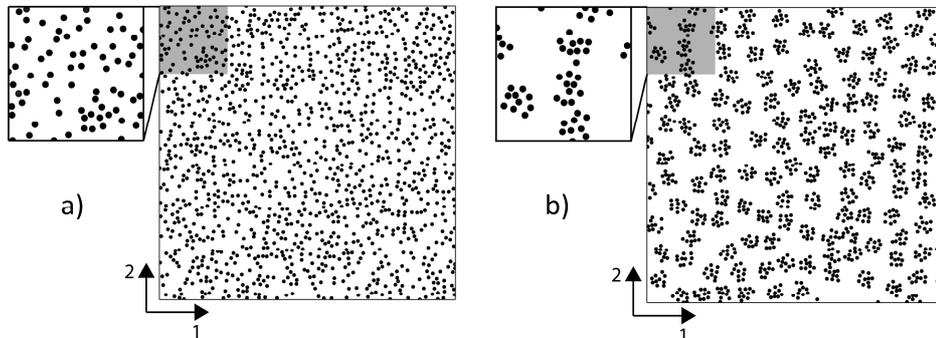
Figure 1: a) Composite microstructure, with uniformly randomly distributed circular inclusions b) Composite microstructure with clustered randomly distributed circular inclusions.
