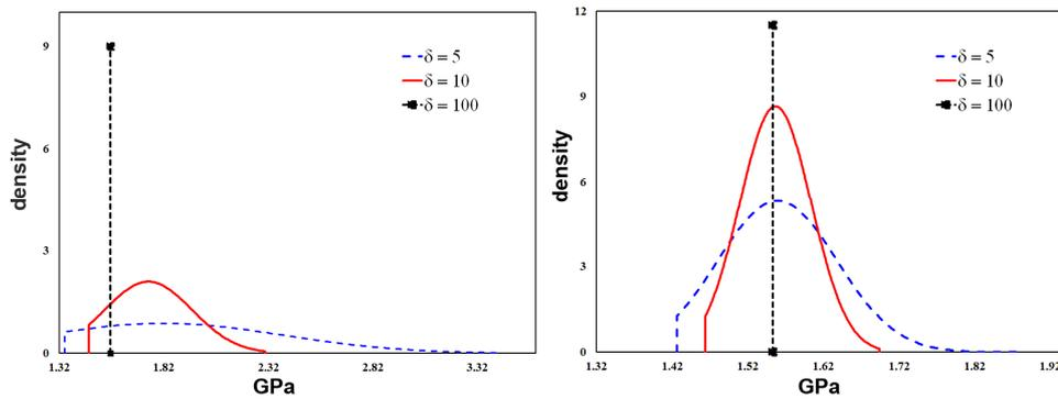
Figure 4: Probability distribution functions for materials with 100:1 contrast ratio. Uniform microstructure with characteristic SVE partition dimensions  $\delta = 5, 10$  and  $100$  is shown. Results are for a) square grid partitioning and b) partitioning by Voronoi tessellation.
