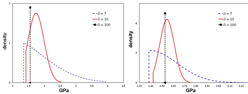
Figure 6: Probability distribution functions for materials with 100:1 contrast ratio. Clustered microstructure with characteristic SVE partition dimensions  $\delta = 5, 10$  and  $100$  is shown. Results are for a) square grid partitioning and b) partitioning by Voronoi tessellation.
