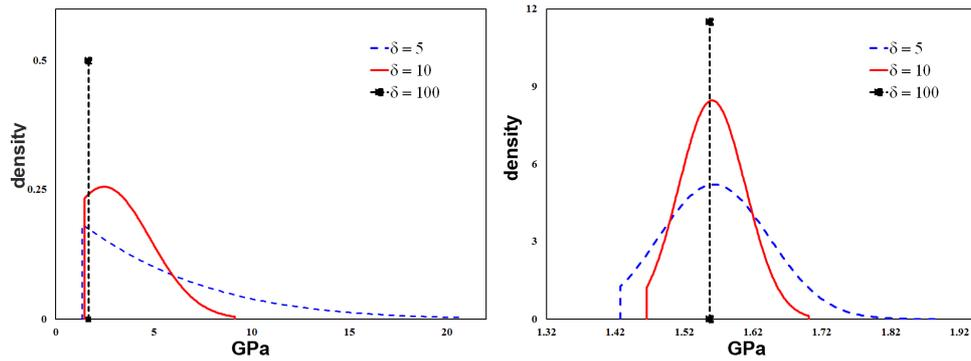
Figure 5: Probability distribution functions for materials with 1000:1 contrast ratio. Uniform microstructure with characteristic SVE partition dimensions  $\delta = 5, 10$  and  $100$  is shown. Results are for a) square grid partitioning and b) partitioning by Voronoi tessellation.
