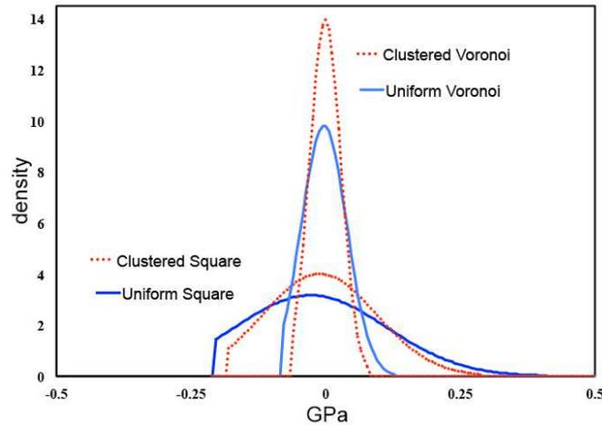
Figure 7: Probability distribution functions based on uniform and clustered microstructures. Zero mean field distributions are shown for comparison. Contrast ratio is 100:1, and characteristic SVE partition dimension is  $\delta = 10$ . Results are given for square grid partitioning and partitioning by Voronoi tessellation.
