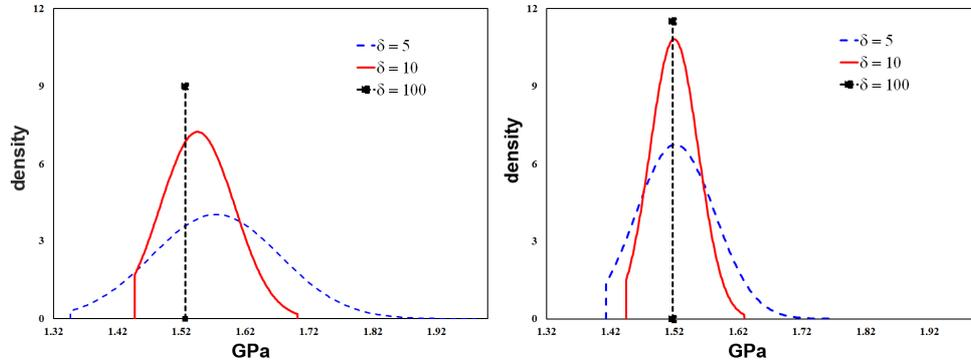
Figure 3: Probability distribution functions for materials with 10:1 contrast ratio. Uniform microstructure with characteristic SVE partition dimensions  $\delta = 5, 10$  and  $100$  is shown. Results are for a) square grid partitioning, and b) partitioning by Voronoi tessellation.
