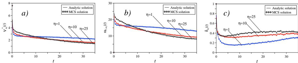
Figure 3: Comparison between the time-variant histories of a) the mean frequency  $\nu_{u_3}^+(t)$  b) the central frequency  $\omega_{C,u_3}(t)$  and c) the bandwidth parameter  $\delta_{u_3}(t)$ , of the third relative to ground floor displacement, by applying the proposed analytical solution and the Monte Carlo Simulation.
