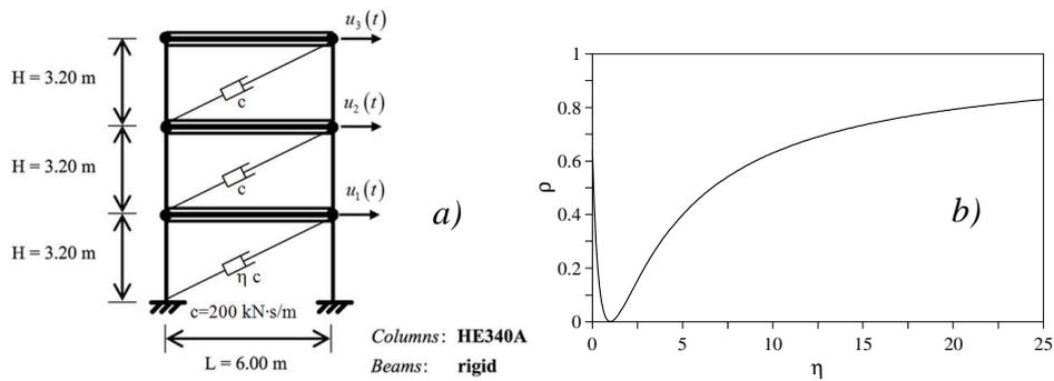
Figure 2: a) Geometric configuration of benchmark three-storey one-bay shear-type frame; b) Coupling index
