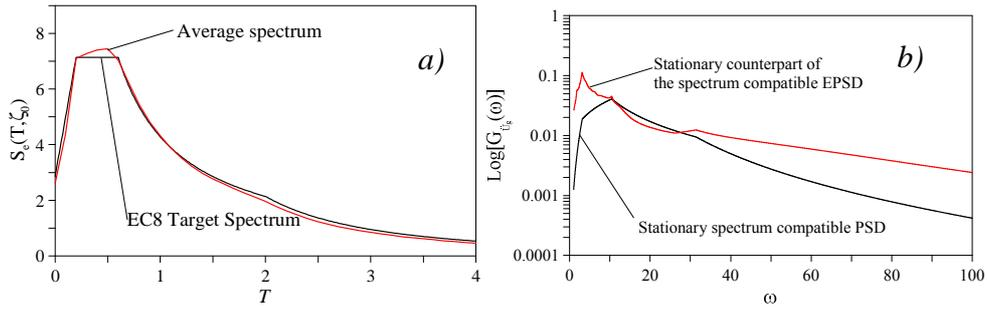
Figure 1: a) Comparison between the selected EC8 target pseudo-acceleration spectrum (black line) and the average of 1000 pseudo-acceleration spectra (red line); b) Spectrum-compatible PSDs. Stationary assumption (black line) and stationary counterpart in the fully non-stationary assumption (red line).
