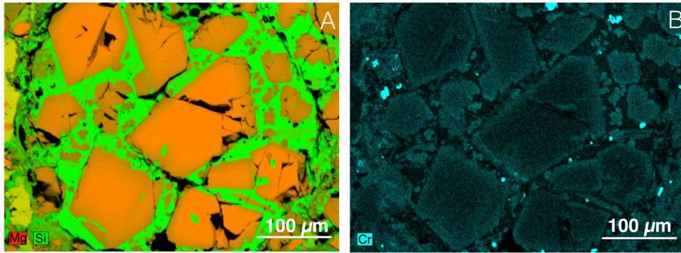
Fig. 4. EDX maps of (A) Si + Mg and (B) Cr in euhedral ferroan olivine grains in a type-II chondrule of Piancaldoli. Olivine rims are enriched in Cr, representing an igneous zoning profile.
