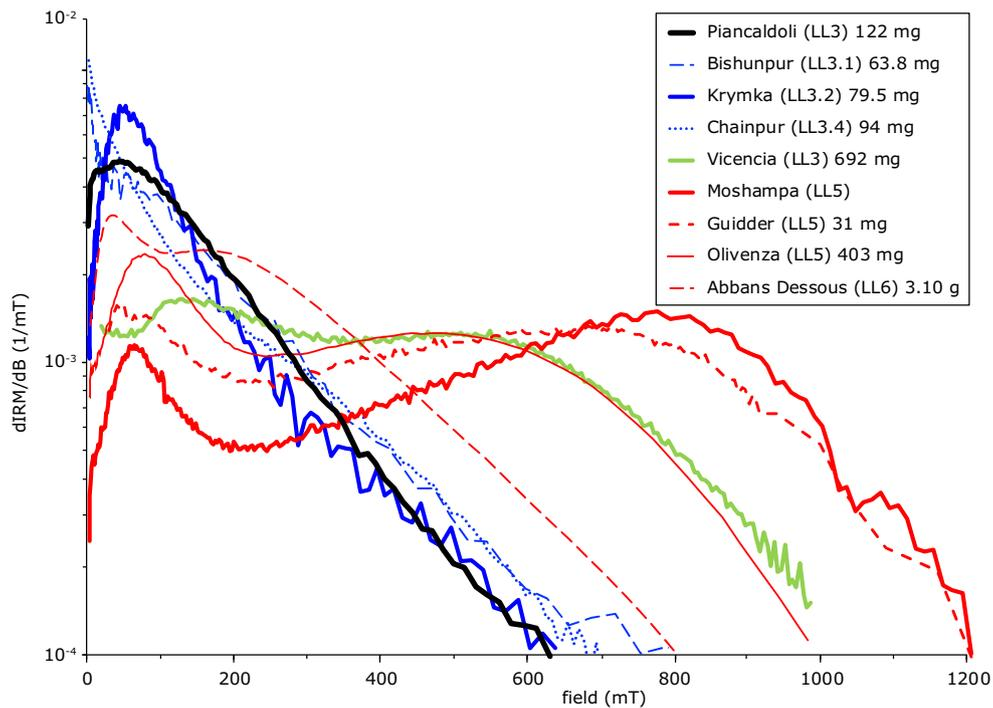
Fig. 10. Coercivity spectra, that is, the derivative of the isothermal remanent magnetization, IRM (normalized to saturation remanence), as a function of the acquisition field, of LL chondrite falls. The petrologic types and masses of each chondrite are indicated.
