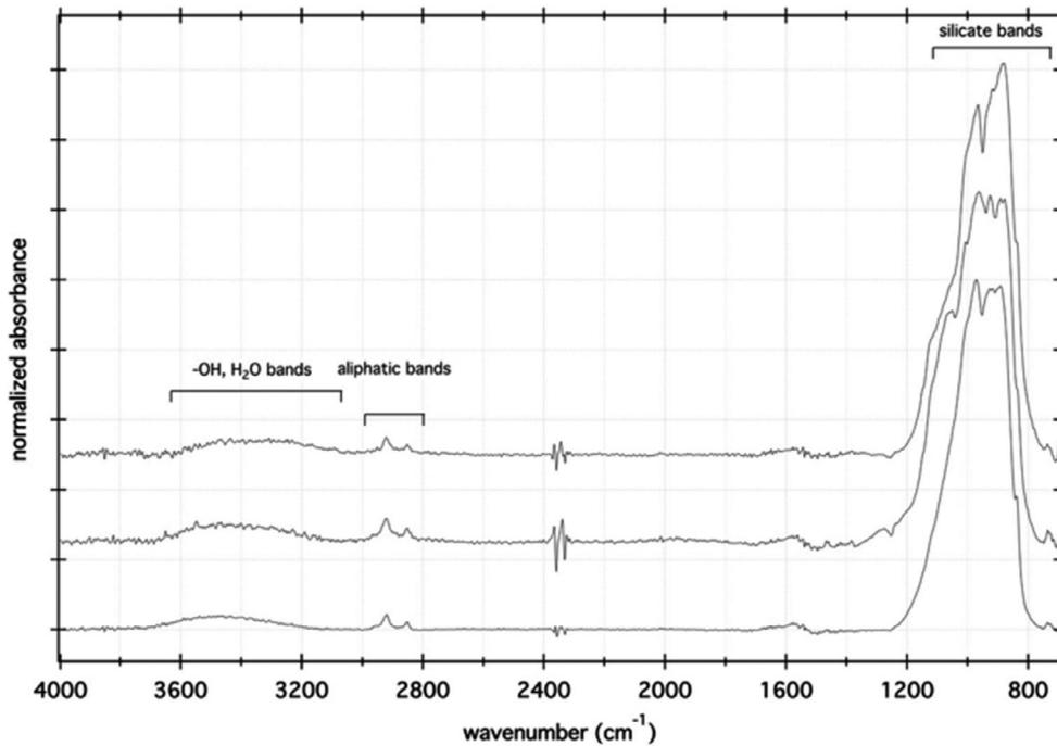
Fig. 8. Baseline-corrected transmission IR spectra (normalized to the height of the Si-O band at  $1000 \text{ cm}^{-1}$ ) of matrix fragments of Piancaldoli, acquired at  $20 \text{ }^\circ\text{C}$  under dynamic vacuum. A vertical offset was applied to ease comparison. Notably, the water band is very weak and olivine is the dominant silicate.
