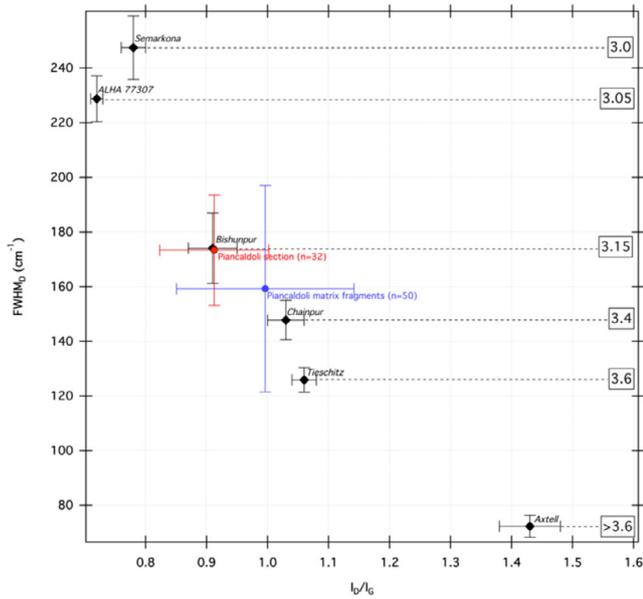
Fig. 7. Spectral parameters (FWHMD versus ID/IG, averages, and one standard deviation) of Raman bands attributed to carbonaceous materials in Piancaldoli compared to other meteorites (see Bonal et al. 2016). Data for Vicencia (LL), Axtell (CV3), and ALHA 77307 (CO<sub>3</sub>) are also reported (see the Magnetic Properties section).
