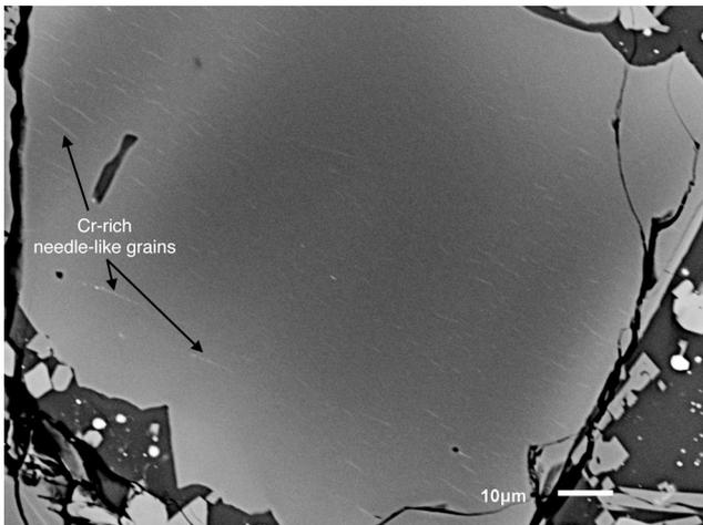
Fig. 5. Backscattered electron image of a ferroan olivine grain in a type II chondrule showing complex, subparallel, needle-like exsolutions of a Cr-rich phase (likely chromite).
