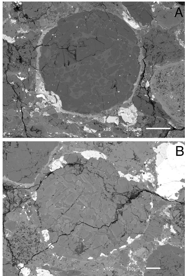
Fig. 2. Backscattered electron images of representative (A) type I and (B) type II chondrules with well-preserved mesostases.
