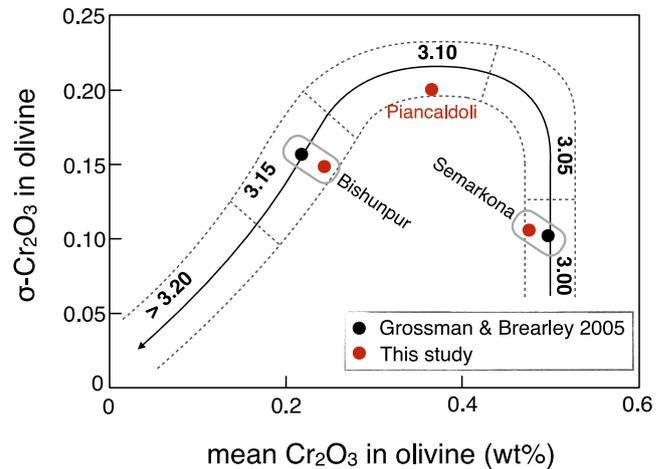
Fig. 6. Standard deviation on  $\text{Cr}_2\text{O}_3$  content versus mean  $\text{Cr}_2\text{O}_3$  content of ferroan olivines in type II chondrules in Piancaldoli compared to Semarkona and Bishunpur (data from this study and Grossman and Brearley 2005). Piancaldoli lies between Semarkona and Bishunpur, suggesting it is of petrologic subtype 3.10.
