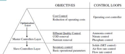
Fig. 3 - Control hierarchy implemented in the A 2 O WWTP.
